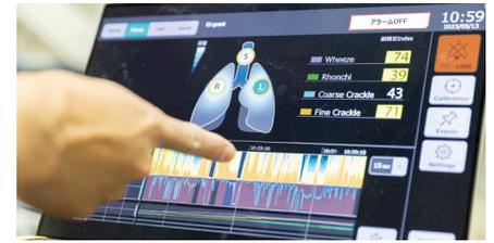
A respiratory sound monitoring system that numerically "visualizes" respiratory sounds, without relying on the skill or auditory sense of physicians and medical staff, was developed in collaboration with a domestic medical device manufacturer. Currently, the system is being developed for monitoring critically ill patients in intensive care units and operating rooms, and for telemedicine for home patients and hotel care patients.
