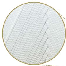
ECMO membrane oxygenator. Venous blood is drained from the body, carbon dioxide, and oxygen are exchanged through thin hollow threads (0.2 to 0.3 mm in outer diameter) with many micropores on the surface and hollow inside, and blood is returned to the body. ECMO replaces the gas exchange function, allowing the inflamed lungs to rest and promoting recovery.
